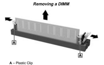
**5.** Store the DIMM in an antistatic bag (available at electronic supply stores) or a cardboard box.
